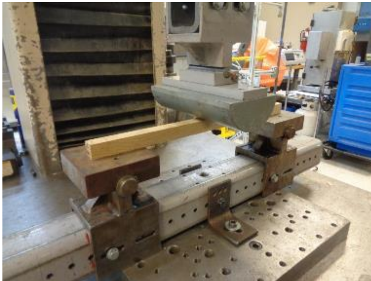
Photo No. 2 ASTM D143, Section 8 Static Bending Test Setup (Wildwood)
