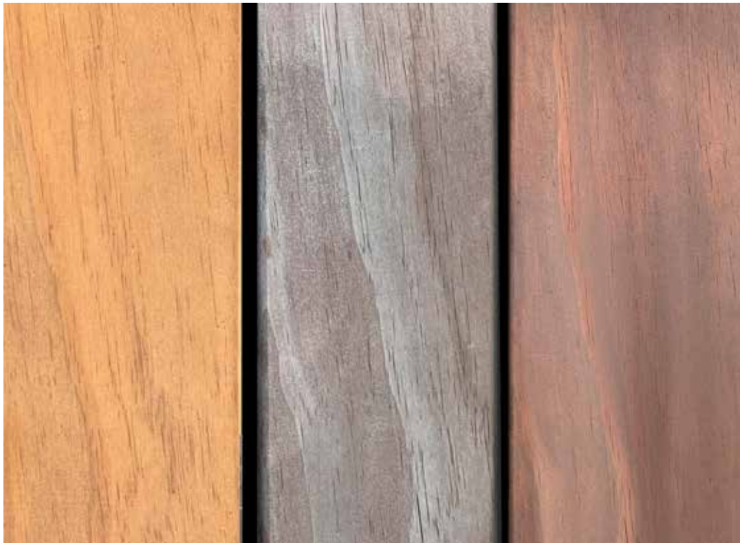
Ticari aged after 2 years installation, no additional oiling
